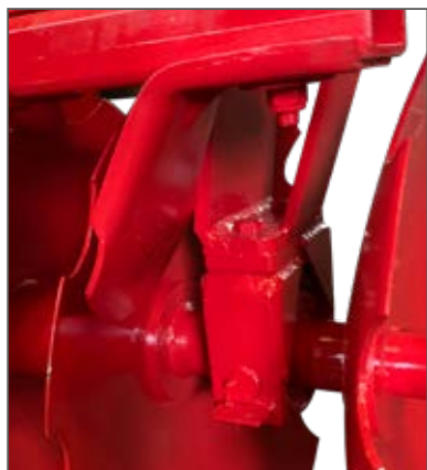
Cuscinetto oscillante Ø 60 a triplice tenuta Oscillating bearing Ø 60 with triple seal
